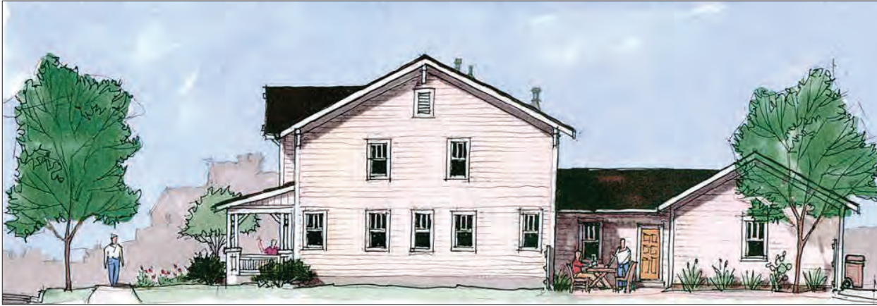
Vents, flues and other roof penetrations should be kept to the rear, out of view from the street.
